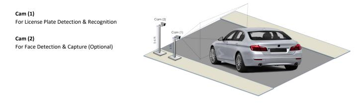
• For Highway: Height of Installation of the Camera is variable and can go up to 25 feet. The angle of Incidence should be between 10 to 40 degrees.
